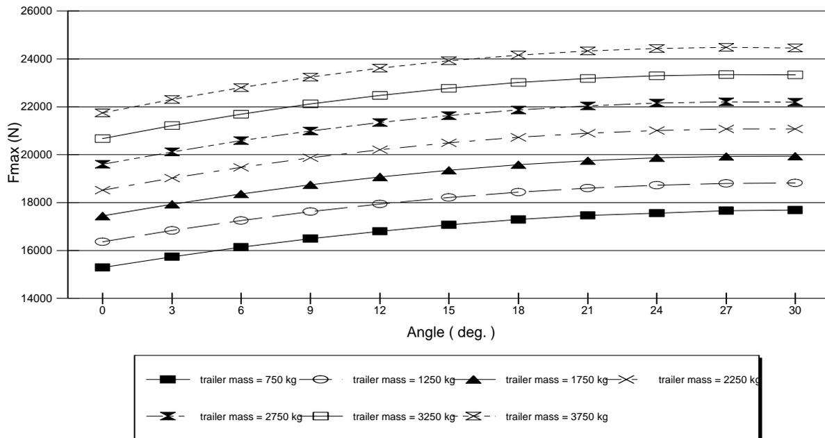
Figure 5. Maximum traction force (F<sub>max</sub>) vs. the slope of the road (uphill) at different total mass of the trailer.
