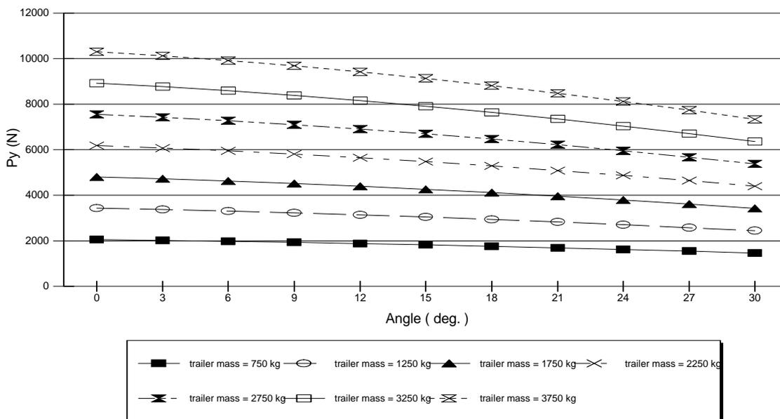
Figure 7. Normal component of the drawbar pull (Py) vs. the slope of the road (uphill) at different total mass of the trailer.
