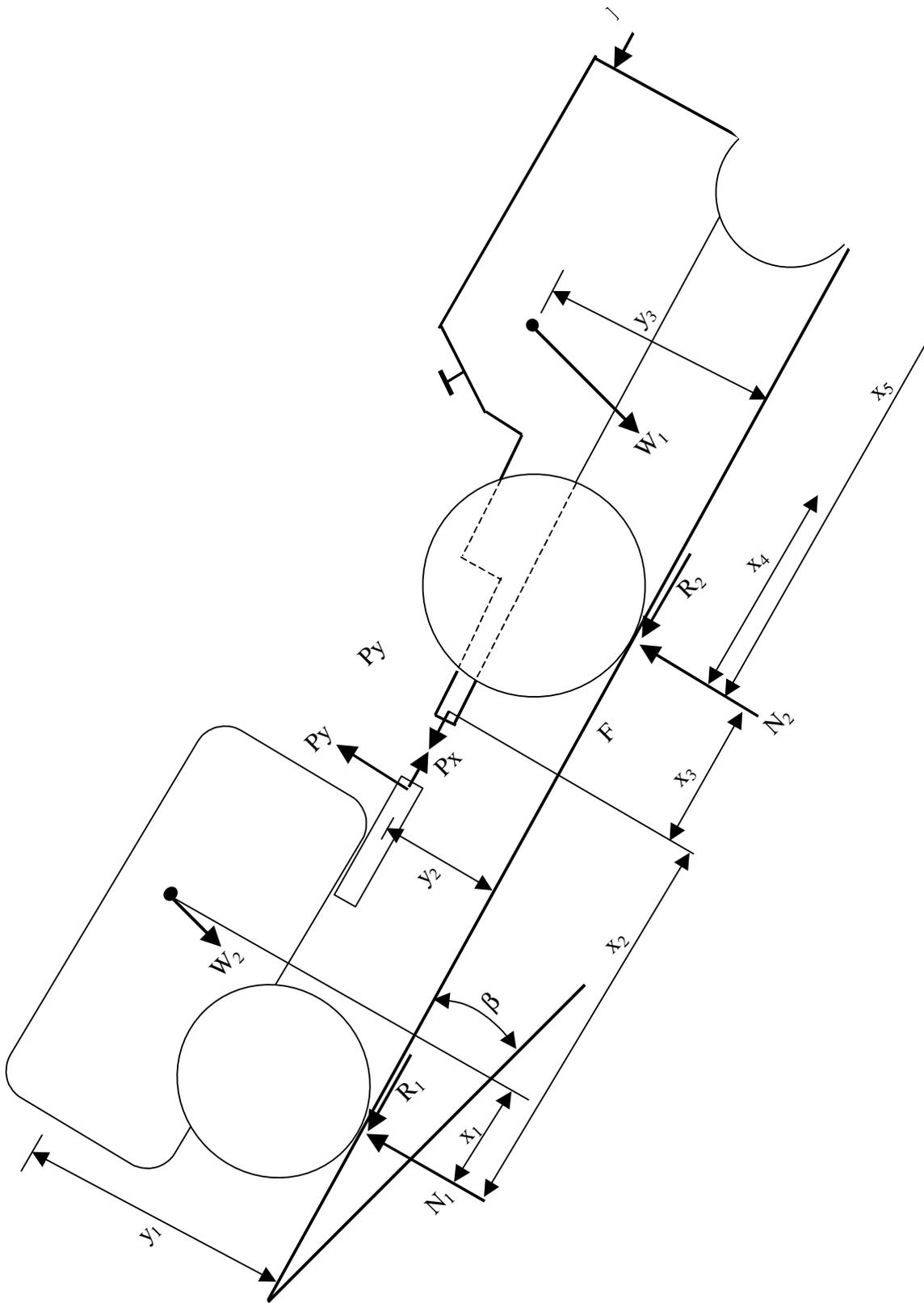
Figure 1. Schematic representation of forces acting on tractor-trailer system.
