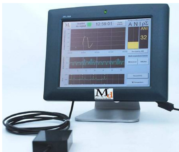
Figure 1 Physiodoloris monitor. Lower scope: ECG signal. Middle scope: normalized, mean centered and band pass filtered RR series. Upper scope: ANI trend curve.
