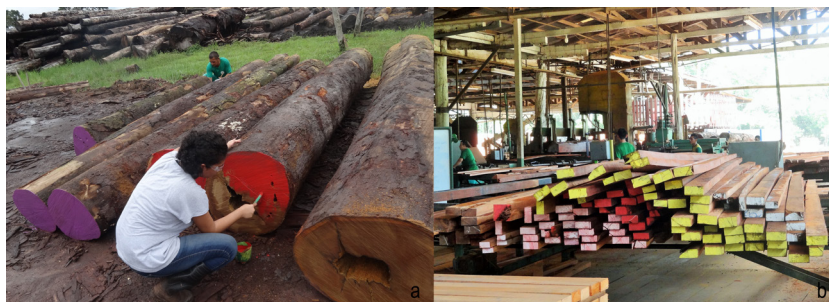
Figure 1. Example of the use of colored water-based ink to mark logs in the sawmill yard (A) for their identification throughout the lumbering process (B). This figure is in color in the electronic version.
