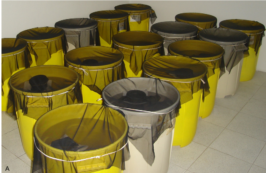
Floating apparatus added to the buckets to separate specimens included at different weeks. A: buckets with the floating apparatus during assay; B: detail of the floating device totally covered with a nylon mesh; C: removal of adult mosquitoes with an aspirator.
