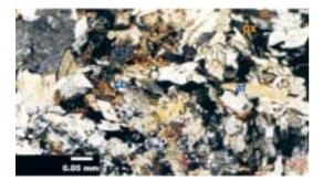
Figure 1. Photomicrograph under transmitted light with crossed polarizers showing crystals of pyroxene (px), amphibole (af), epidote (ep) and carbonate (cb).
