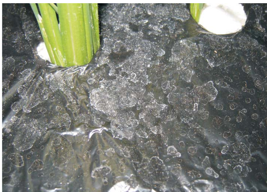
Figure 3. White precipitate on the polyethylene cap that covered the pots with plants.
