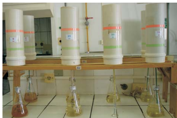
Figure 1. PVC columns with samples of natural soil and soil-sludge mixtures.
