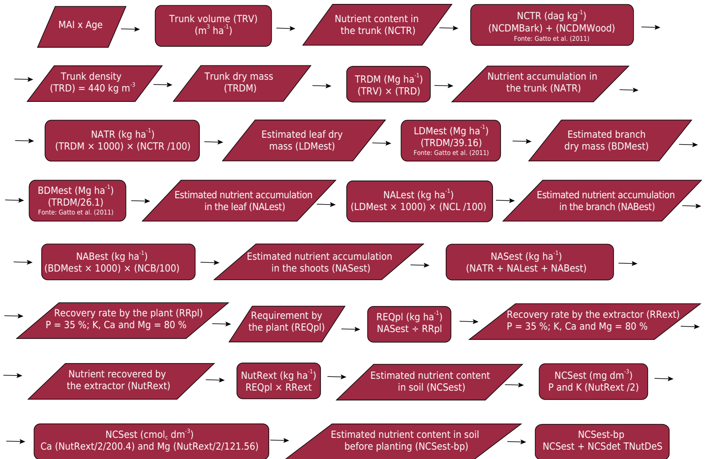
Figure 1. Flowchart of the steps used to obtain the estimated contents of nutrients ( P , K^+ , Ca^{2+} , and Mg^{2+} ) in the soil in the 0.00-0.20 m layer before planting.
