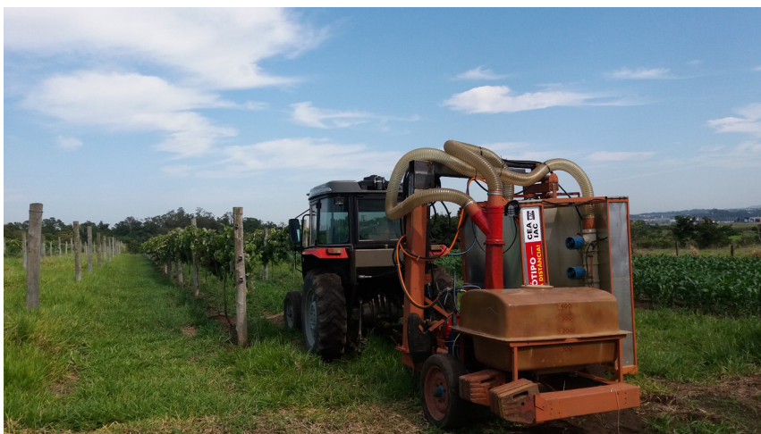
Figure 4. Vineyard operation of the recycling sprayer prototype.
