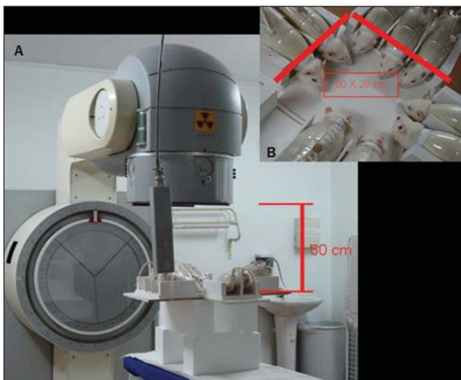
Figure 1. A: Radiotherapy Philips XK 5101 model equipment. Animals placed on the equipment with the head at a 60 cm distance from the radioactive source. B: Animals positioned on a wooden device with slots, inside the plastic restrainer.
