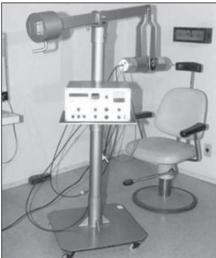
**Figure 3.** SCT-13004 scintillation probe of the HUCFF-UFRJ Division of Nuclear Medicine.
