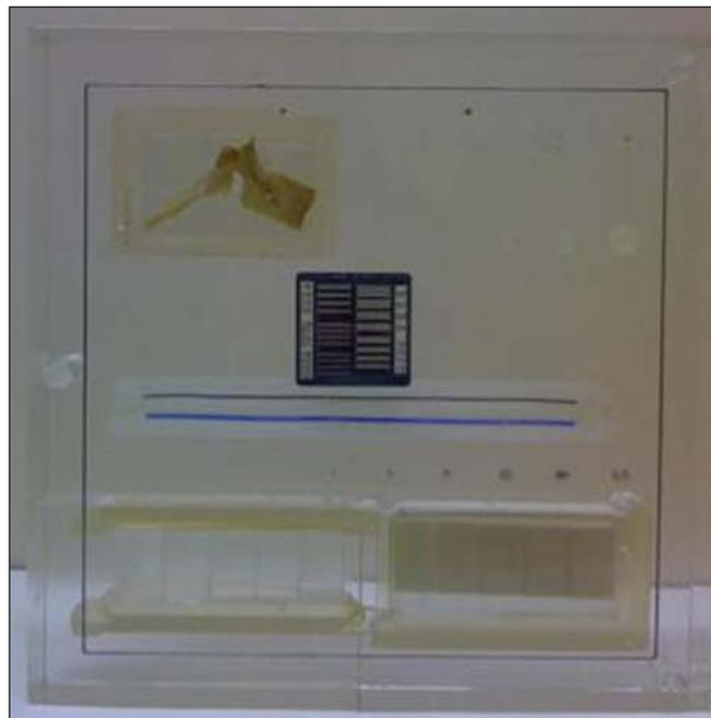
**Figure 2.** Realistic-analytic phantom adapted for fluoroscopy.
