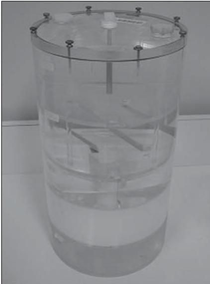
**Figure 2.** Quality phantom for analysis of noise, contrast and spatial resolution of the image.
