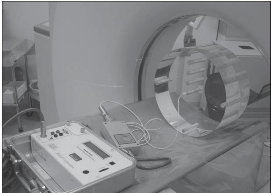
**Figure 1.** Electrometer, ionization chamber and body phantom exposed to the tomographic beam for CTDI calculation.
