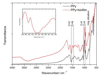
Figura 3. FTIR spectrum of polypyrrole and polypyrrole+ biofilm of S. aureus (in the inset is shown the region around 860 cm<sup>-1</sup> for sample PPy+biofilm)
