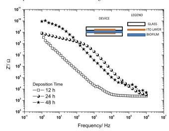
Figure 4. Real part of impedance of biofilms deposited on ITO layers/ glass substrates
