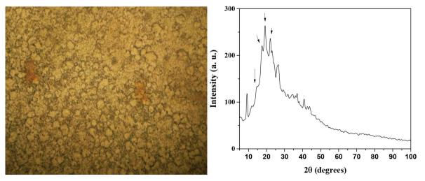
Figure 1. A) Image of optical microscopy (4X), B) X ray diffraction patterns of polysaccharides extracted from Persea americana var. Hass avocado seeds
