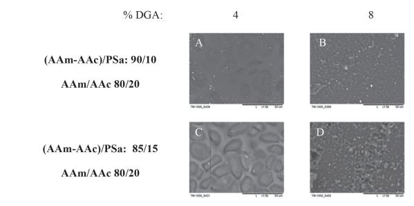
Figure 7. SEM micrographs for xerogels synthesized via photoinitiated polymerization, with 10 and 15 wt. % of polysaccharides (AAm-AAc / PSa: 90/10 and 85/15 respectively) and 4 and 8 wt. % DGA relative to acrylic monomers
