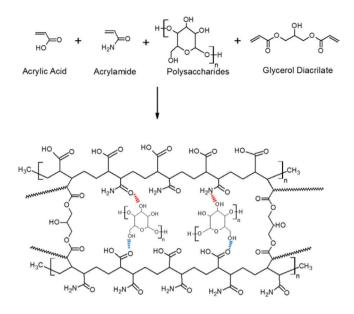
Figure 2. Schematic representation of acrylic hydrogels with polysaccharides
