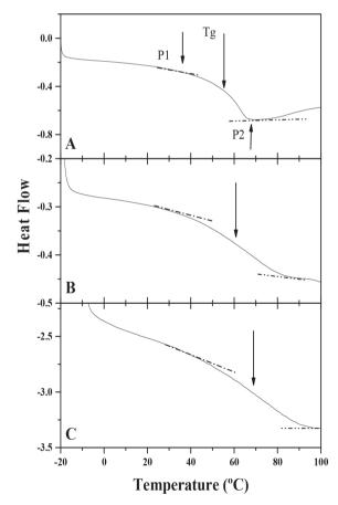
Figure 5. DSC of: A) AAm (8% DGA), B) AAc (8%DGA), C) PSa
