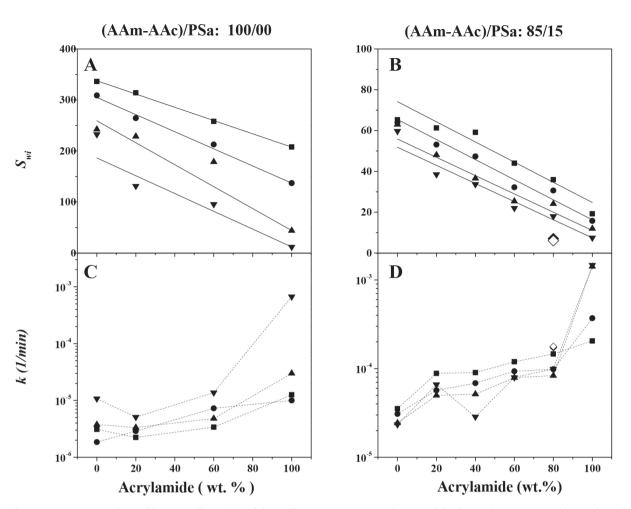
*Figure 10. Kinetic parameters: the equilibrium swelling* ( $S_{wi}$ ) *and the swelling rate constant as a function of the chemical composition without polysaccharide* (A, B) *and with polysaccharide* (C, D) *for hydrogels synthesized via redox polymerization.* ( $\blacklozenge$ ) *and* ( $\diamondsuit$ ) *represent values obtained for hydrogels synthesized via photoinitiated polymerization with 4 and 8 wt. % of DGA respectively*
