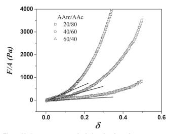
Figure 11. Stress-strain curves for hydrogels subjected to compression measurements
