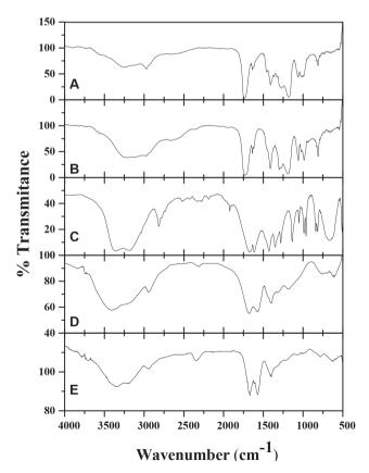
Figure 4. FTIR spectra of: A) AAc, B) GDA, C) AAm, D) copolymer AAm/ AAc (40/60), with 4 wt. % GDA, and E) copolymer of AAm/AAc 50/50 with 8 wt. % GDA and 15 wt. % PSa; (AAm-AAc)/PSa: 85/15
