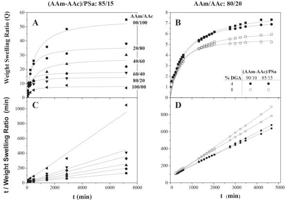
Figure 9. Swelling kinetics of hydrogels with polysaccharide for several AAm/AAc ratios synthesized via redox polymerization (A and C) and photoinitiated polymerization (B and D)
