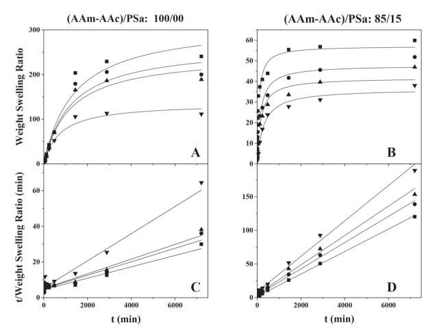
*Figure 8.* Swelling kinetics of hydrogels without polysaccharide (A and C) and with polysaccharide (B and D) with a ratio of acrylic monomers AAm/AAc 20/80 for different concentrations of DGA,  $(\blacksquare)$  0.5,  $(\bullet)$  1,  $(\blacktriangle)$  4 y  $(\bigtriangledown)$  8 wt. % relative to acrylic monomers
