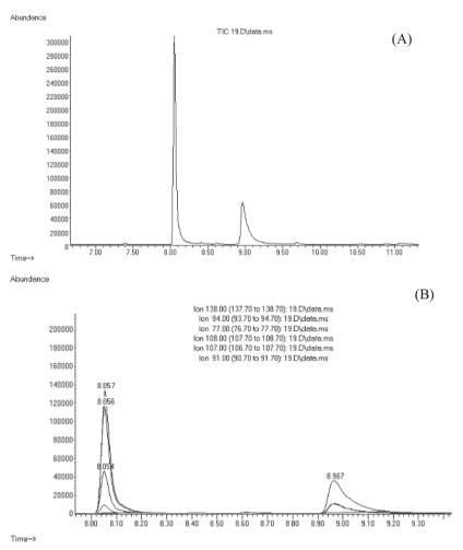
Figure 1. A. Total Ion Chromatogram of an ink sample from the Factorial Project (assay 19), showing 2-PE peak at RT 8.96, and Internal Standard peak at RT 8.05. B. Extracted ion chromatogram of the same sample, showing the main ions of 2-PE and Internal Standard
