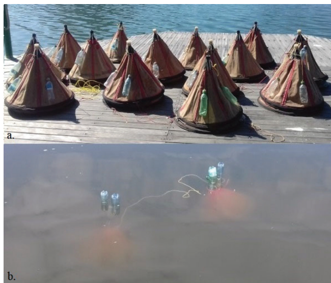
Figure 2. “Inverted” funnels used to collect methane ebullitive flux. a. funnels before being placed in the water; b. two funnels tied together in the water attached to anchors to be placed in the correct depth and the apex connected to a collection flask
