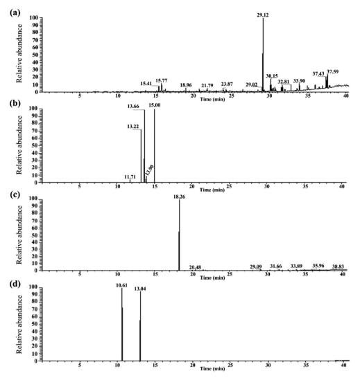
Figure 5. Total ion chromatogram. a) Raw sanitary landfill leachate, b) first stage of Fenton process, c) second stage of Fenton process and d) third stage of Fenton process
