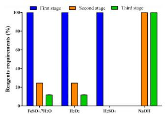
Figure 3. Comparison of reagents requirements among the three stages of Fenton process.  $Fe_2SO_4$ .  $7H_2O$ : ferrous sulfate heptahydrate;  $H_2O_2$ : hydrogen peroxide;  $H_2SO_4$ : sulfuric acid; NaOH: sodium hydroxide
