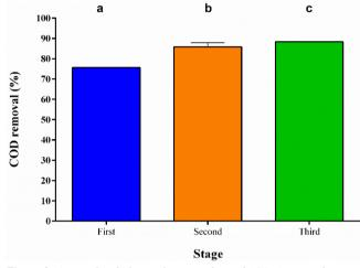
Figure 2. Accumulated chemical oxygen demand (COD) removal corresponding to each stage of Fenton process. Different letters indicate statistical differences (p < 0.05) according to an LSD test
