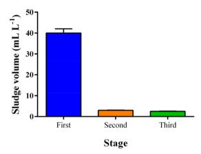
Figure 4. Sludge production in each stage of Fenton process
