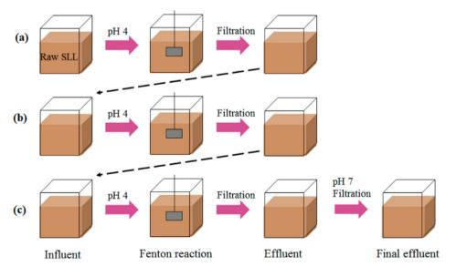
Figure 1. Experimental setup of the triple-stage Fenton process: a) first stage, b) second stage and c) third stage. SSL: Sanitary landfill leachate
