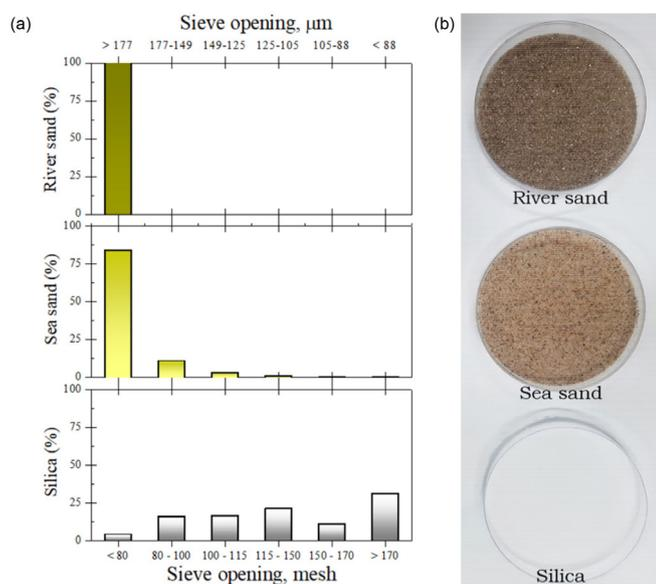
**Figure 10.** (a) Granulometric studies by sieving the materials used as stationary phases in chromatographic separation of the food coloring; (b) photography of each studied material
