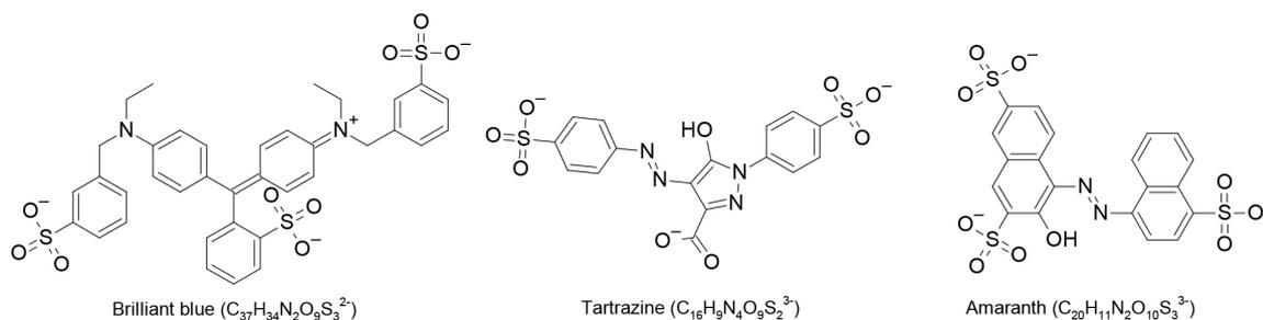
**Figure 1.** The chemical structures of the dyes constituting the dark brown food coloring powder, according to the information displayed in product's label. All compounds are sodium salts
