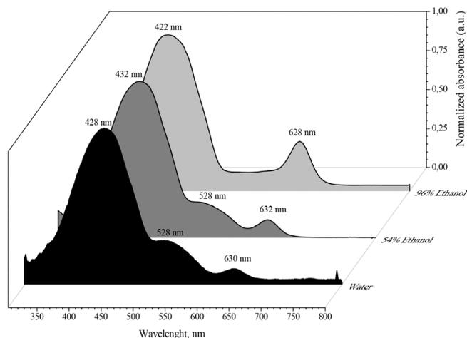
**Figure 3.** Electronic spectra of the food coloring in 96% ethanol, 54% ethanol and water (for color solutions, see Figure 2)
