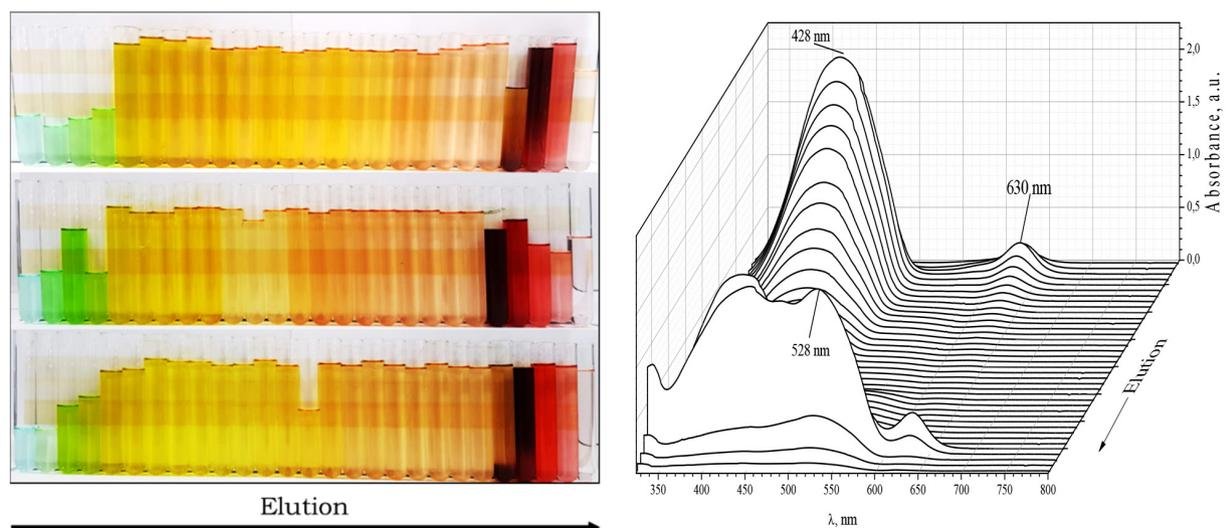
**Figure 8.** Left: fractions collected during the experiment using sea sand as a stationary phase (in triplicate); Right: spectra registered for all fractions collected. All experiments were run in the handmade chromatographic column and all the spectra were recorded in water
