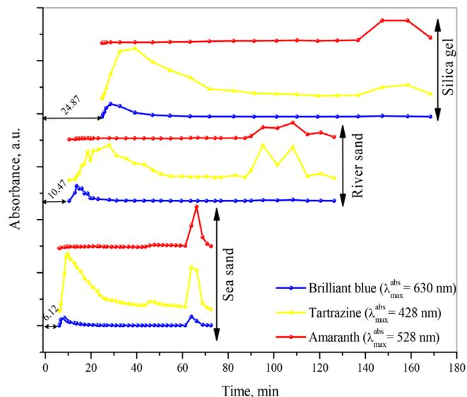
**Figure 5.** Chromatograms constructed from spectrophotometric measurements for each stationary phase studied
