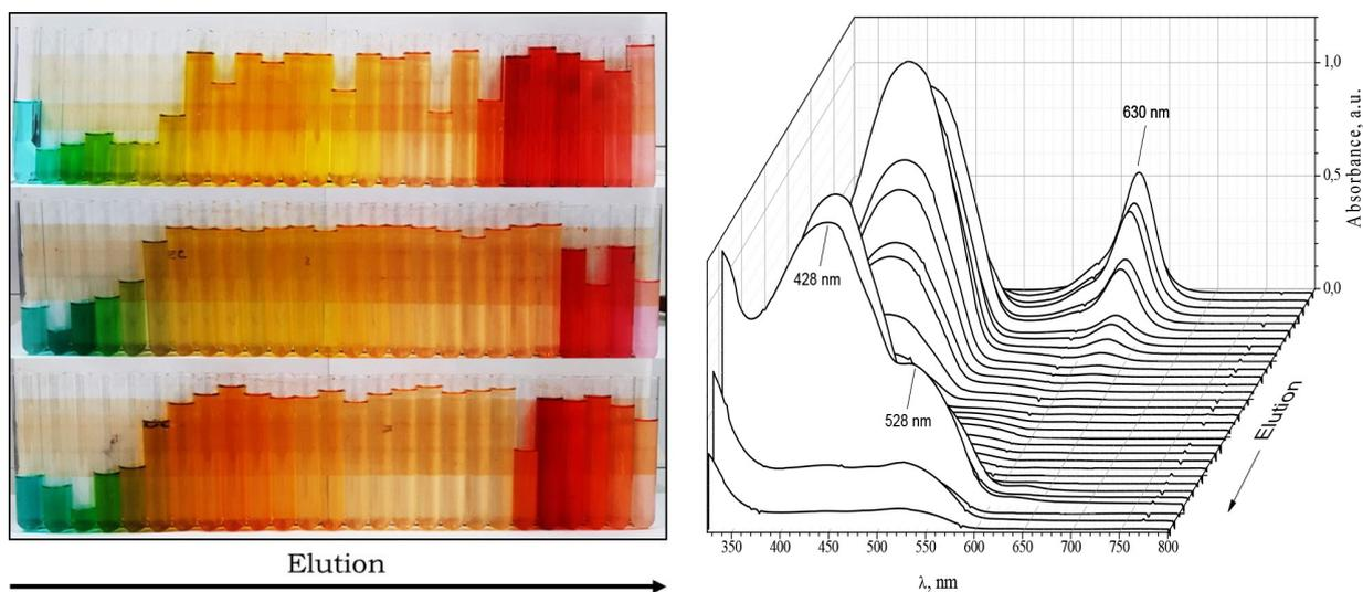
**Figure 7.** Left: fractions collected during the experiment using river sand as a stationary phase (in triplicate); Right: spectra registered for all fractions collected. All experiments were run in the handmade chromatographic column and all the spectra were recorded in water
