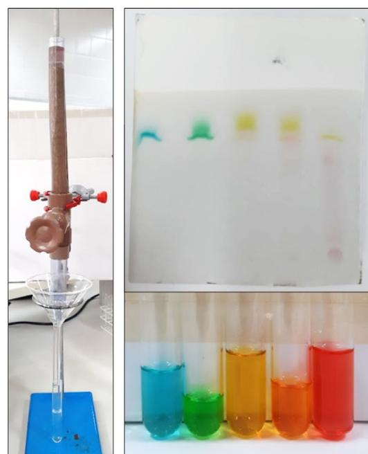
**Figure 4.** Column chromatography experiment using the handmade column and river sand as a stationary phase. Some tube tests of collected fractions are shown as well as the corresponding silica TLC analyses for each fraction using 96% ethanol solution as eluent
