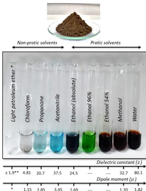
**Figure 2.** Food coloring (above) and food coloring solubility test in protic and non-protic solvents (below). \*Dipole moment value not found for that substance; \*\*Value attributed from n-hexane<sup>24</sup>
