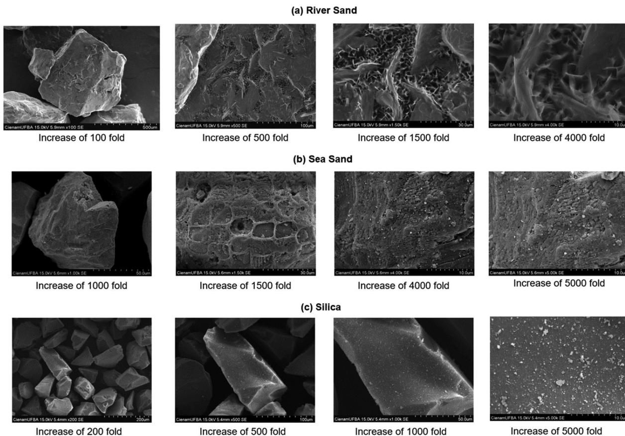
**Figure 11.** SEM images with different magnifications for the adsorbents studied
