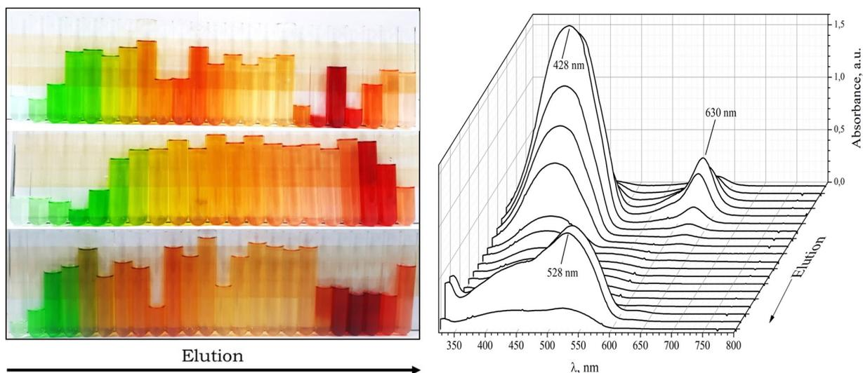
**Figure 6.** Left: fractions collected during the experiment using silica as a stationary phase (in triplicate); Right: spectra registered for all fractions collected. All experiments were run in the handmade chromatographic column and all the spectra were recorded in water
