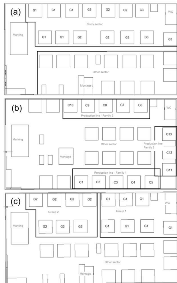
Figure 2 – Representation of the layout currently used by the studied industry (a), alternative scenario 1, linear layout (b) and alternative scenario 2, process layout (c).
