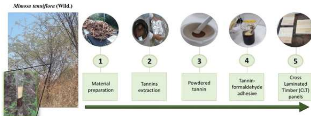
Figure 1 – Schematic representation of the stages for assessing the quality of cross-laminated timber panels bonded with an adhesive based on tannins from M. tenuiflora bark.
