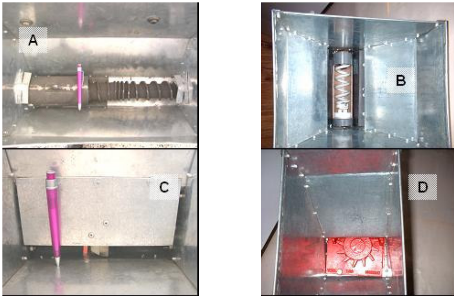
FIGURE 1. Fertilizer metering systems evaluated: A-Feed screw; B-wire auger; C-ridged traction wheels; D-star-shaped feed wheel.
