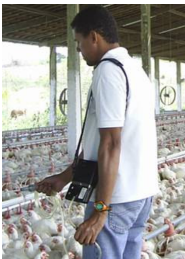
FIGURA 3. Monitor de gases portátil digital (PHD5 Biosystems®). Digital portable gas monitor (PHD5 Biosystems®).
