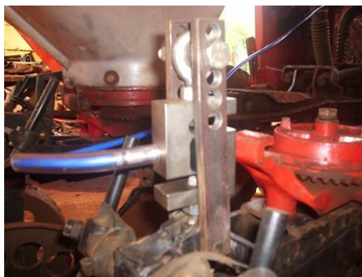
FIGURE 1. Location of the load cell in the seeder-fertilizer.
