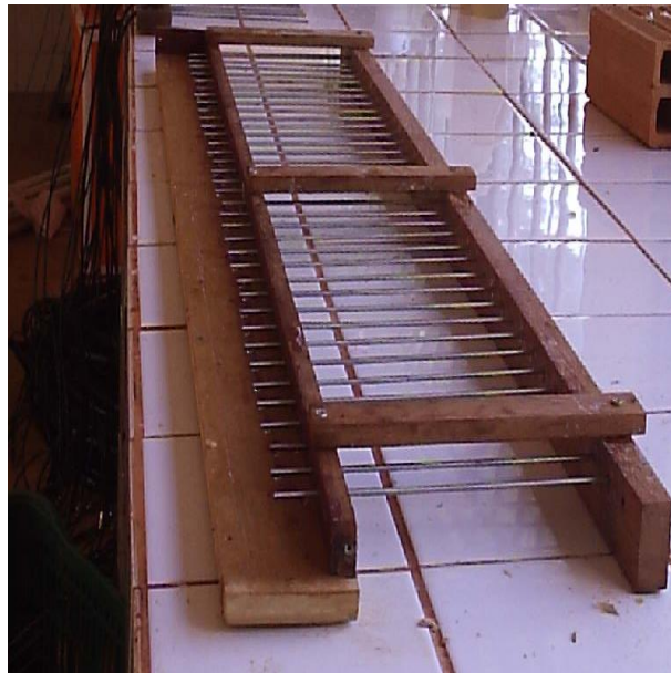
FIGURE 1. Wood template with parallel rods of stainless steel, separated by 0.02 meters, constructed for assembly of TDR probes.
