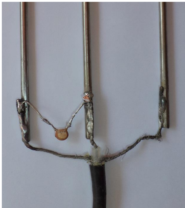
FIGURE 2. Structure of TDR probes built at the Laboratory of Water Resources and Environmental Sanitation of the State University of West Paraná (UNIOESTE), Campus of Cascavel city, state of Paraná (PR), Brazil.
