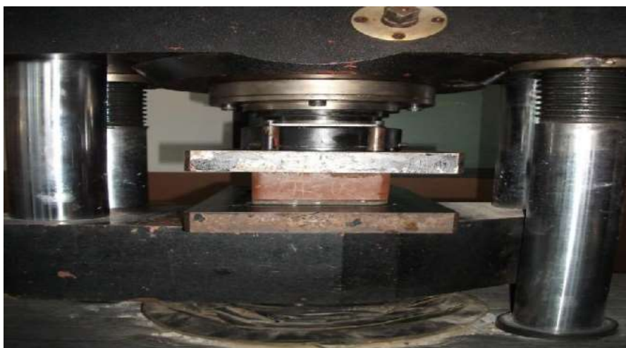
FIGURE 4. Compressive strength test1
