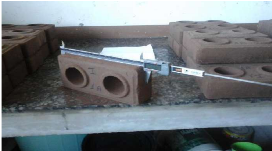
FIGURE 2. Measurement of the bricks according to NBR 10834 (ABNT, 2013b)
