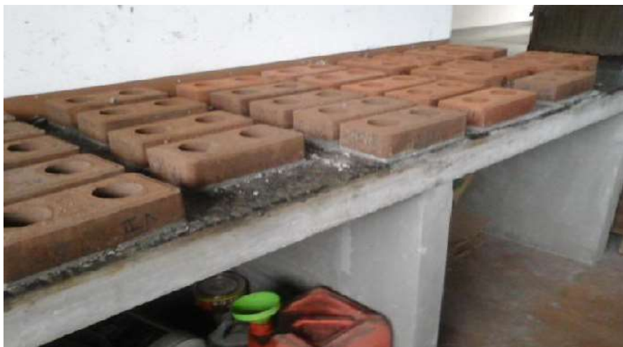
FIGURE 3. Bricks capped with Portland cement paste.
