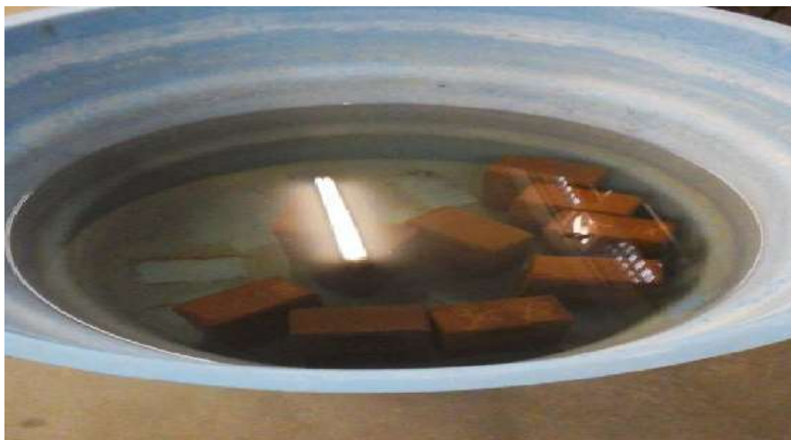
FIGURE 5. Bricks immersed in water to perform the absorption test.
