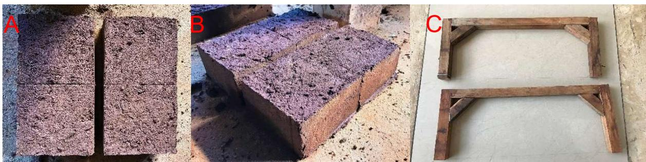
Top view of the adobes cut after the demolding (A), side view of the adobes cut after the demolding and (B) apparatus created to cut the adobes (C). FIGURE 4. Methodology proposed to cut the adobe for the compression test.
