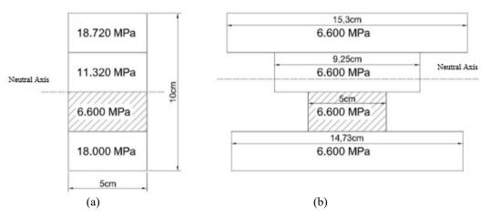
FIGURE 2. Geometry and MOE of the composed elements of the beam: (a) original section; (b) transformed section.
