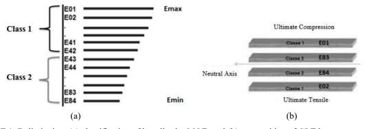
FIGURE 1. Delimitation: (a) classification of lamellae by MOE, and (b) composition of GLT beams.
