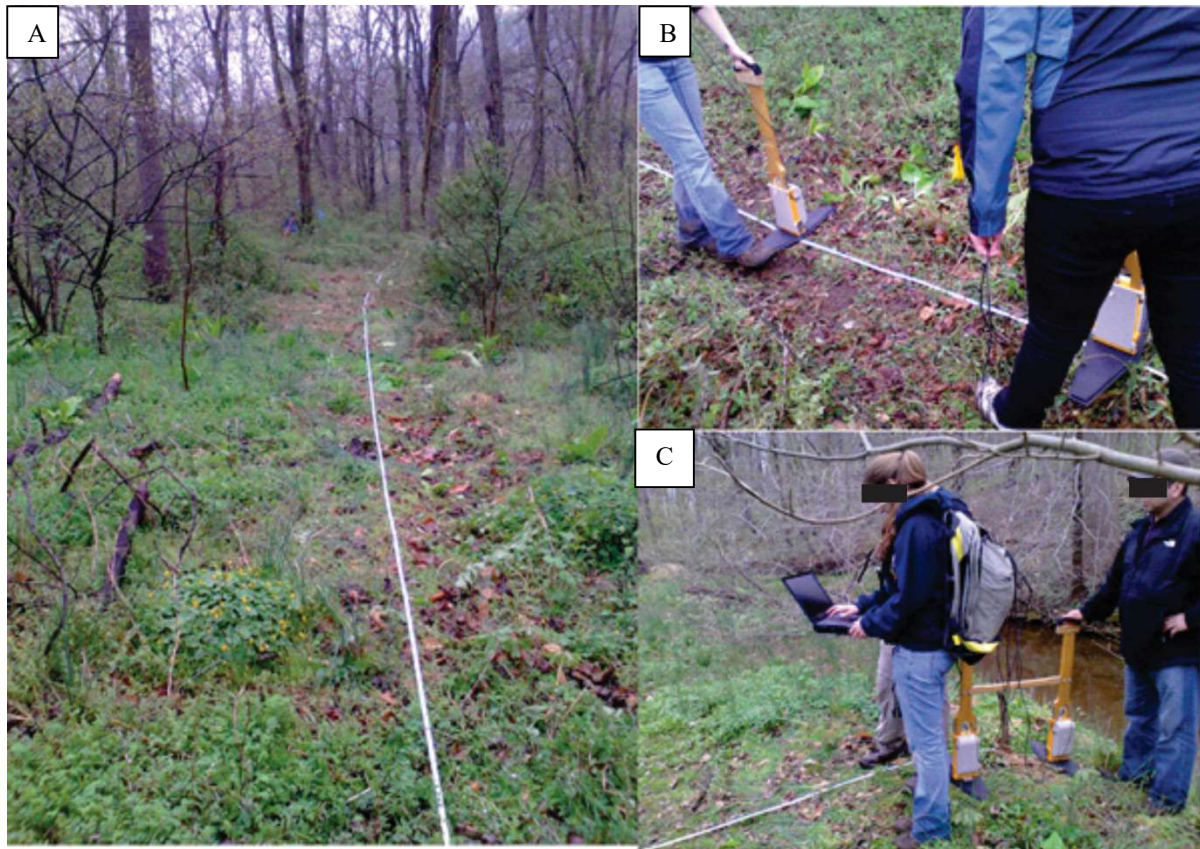
FIGURE 2. Field campaign in the Elizabeth Creek watershed in New Jersey, USA. A) Location where measurements were completed using GPR; B) Measurements using the CMP method; and C) Measurements using the COP method.
