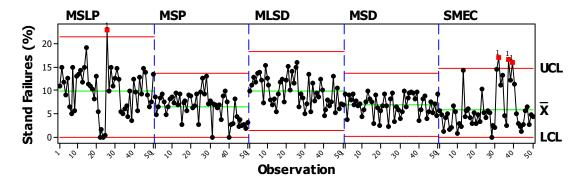
FIGURE 3. Control charts for stand failures at 90 days after planting for operation quality of sugarcane planting. MSLP: mechanized strawless planting; MSP: mechanized straw planting; MSLD: mechanized strawless distribution; MSD: mechanized straw distribution; SMEC: semi-mechanized planting. UCL: upper control limit; LCL: lower control limit; X: means of individual values.
