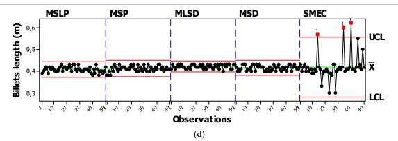
FIGURE 1. Control charts for the variables for sugarcane planting: number of gems  $m^{-1}$  (a); number of viable gems  $m^{-1}$  (b); number of unviable gems  $m^{-1}$  (c); and billets length (d).
