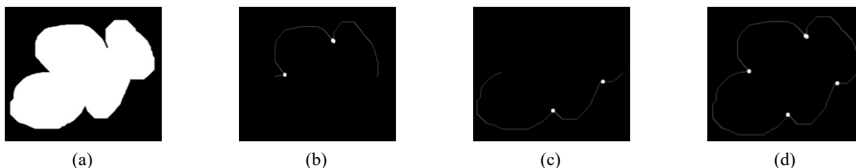
FIGURE 10. Segmentation points for region No.13. (a) binary image, (b) first two segment points, (c) last two segment points, and (d) all segment points on the edge.
