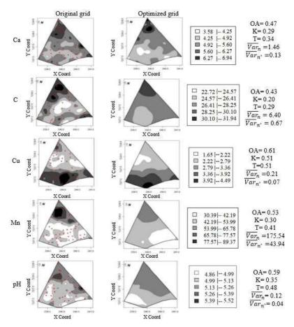
FIGURE 5. Thematic maps of soil chemical attributes constructed with the original and optimized sampling grid. • represents each selected location in the original grid to compose the optimized grid. Estimated values of OA (overall accuracy), K, and T (Tau and Kappa concordance indices), mean of kriging variance of the original configuration ( $\overline{Var}_n$ ) and of the optimized ( $\overline{Var}_{n^*}$ ).
