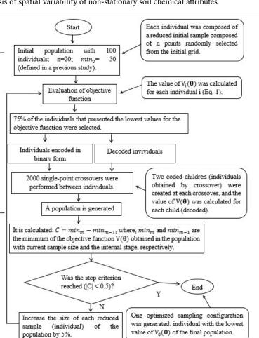
FIGURE 2. Flowchart of the optimization process of configuration and sample size.
