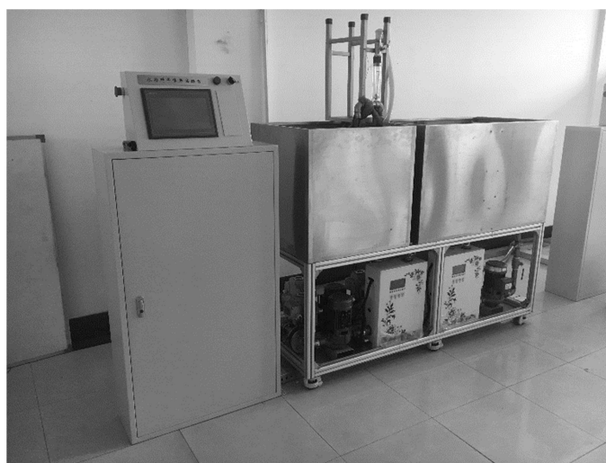
FIGURE 8 Rice seed soaking and germination device.
