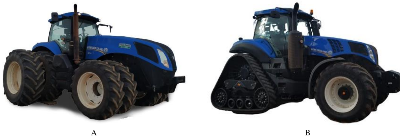
FIGURE 1. Tractors used in the experiment; (A) tractor equipped with wheels on the front and rear axles and (B) tractor equipped with single wheels on the front axle and half-track on the rear axle. Espigão do Leste, MT, Brazil, 2019.
