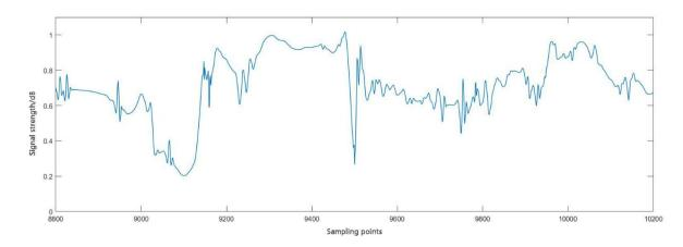
FIGURE 7. Waveform of acceleration signal de-noised using wavelet soft threshold function.
