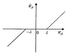
FIGURE 4. The diagram of soft-thresholding function.
