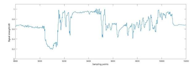
FIGURE 10. Waveform of acceleration signal de-noised using wavelet improved threshold function.
