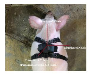
FIGURE 1. Direction of the back-mounted triaxial accelerometer. The X-axis pointed from the left to the right side of the pig's body, the Y-axis pointed from the tail to the head of the pig, and the Z-axis was perpendicular to the XY plane.
