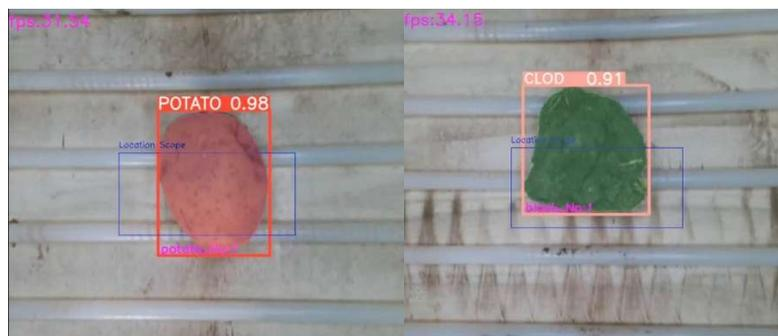
(a) All potatoes and clods are identified under the lower conveying speed
