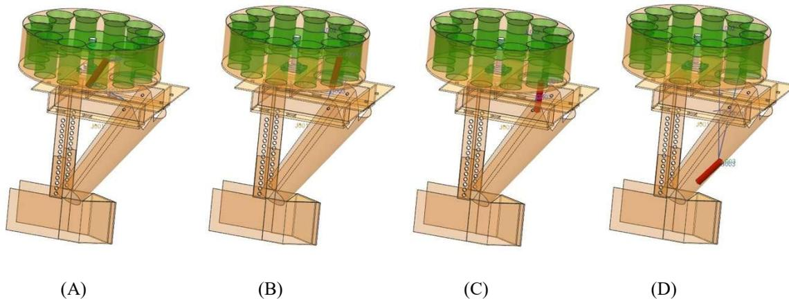
FIGURE 6. The trajectory of cassava stalks in the seeding process. (A) Stalk transfer process. (B) Entering the stalk orifice. (C) Stalk expulsion process. (D) Entering the stalk groove.
