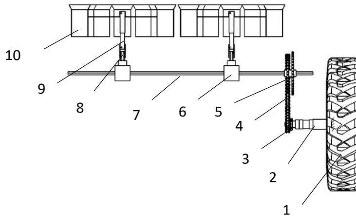
FIGURE 7. Structural diagram of the transmission system: 1) ground wheel; 2) transmission shaft III; 3) driving sprocket; 4) chain; 5) driven sprocket; 6) commutator; 7) transmission shaft II; 8) transmission connection sleeve; 9) transmission shaft I; and 10) stalk cup.
