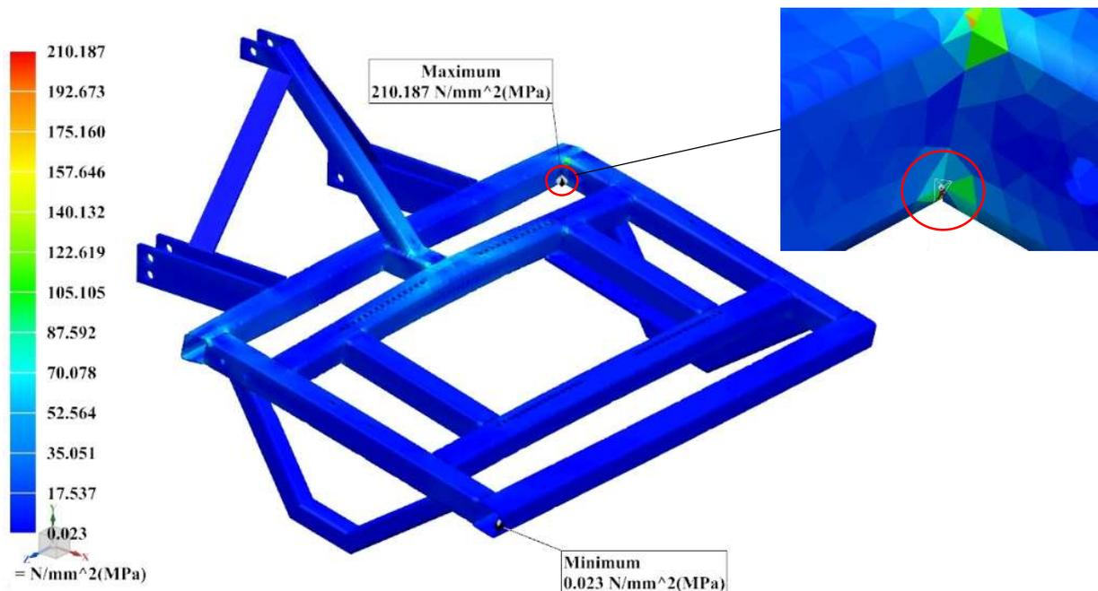
FIGURE 9. Stress cloud of the frame.
