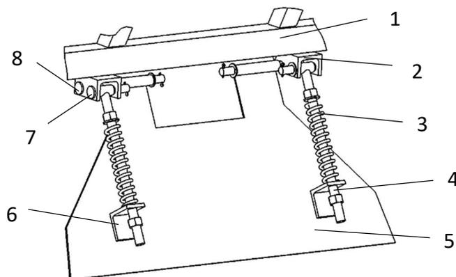
FIGURE 11. Schematic of the soil-covering system: 1) frame; 2) mounting base; 3) coil spring; 4) support rod; 5) soil cover board; 6) location base; 7) support rod positioning dowel; and 8) cover board positioning dowel.
