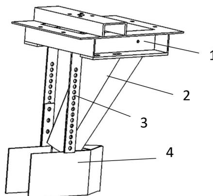
FIGURE 10. Schematic of the gatherer and furrow opener system: 1) positioning frame; 2) gatherer; 3) height adjusting plate; and 4) furrow opener.
