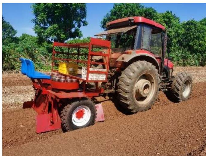
FIGURE 12. Trials for the rotary dibble-type cassava planter.
