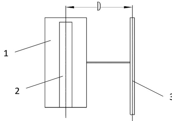
FIGURE 5. Schematic diagram of cassava stalk position: 1) stalk cup; 2) cassava stalk; 3) transmission shaft I; and D) the distance between the cassava stalk and the centerline of the metering device.
