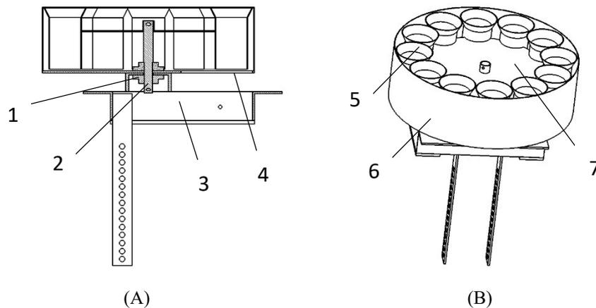
FIGURE 4. Structural diagram of the metering device: 1) bearing housing; 2) transmission shaft I; 3) clamping frame; 4) stalk orifice; 5) stalk cup; 6) protective cover; and 7) connecting plate of the stalk cup. (A) Front view. (B) Isometric view.
