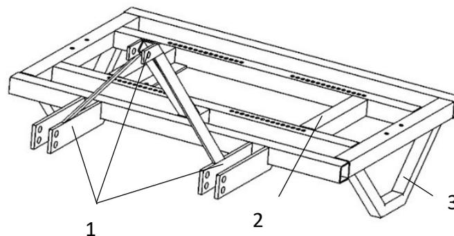
FIGURE 8. Structure of the frame: 1) three-point hitch; 2) upper frame; and 3) lower frame.
