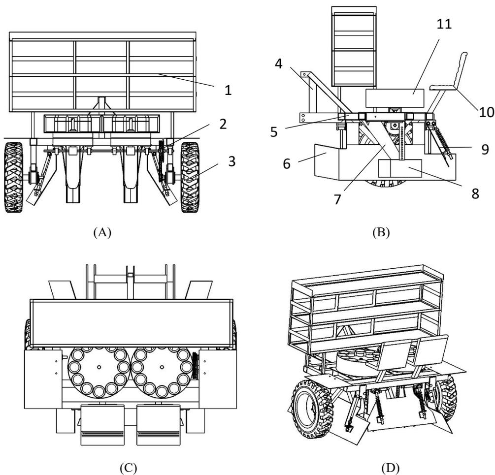
FIGURE 3. Structural diagram of a rotary dibble-type cassava planter: 1) cassava stalk box; 2) transmission system; 3) ground wheel; 4) three-point hitch; 5) frame; 6) ridge plate; 7) stalk groove; 8) furrow opener; 9) soil-covering system; 10) seat; and 11) rotary dibble-type stalk metering device. (A) Front view. (B) Right view. (C) Top view. (D) Isometric view.
