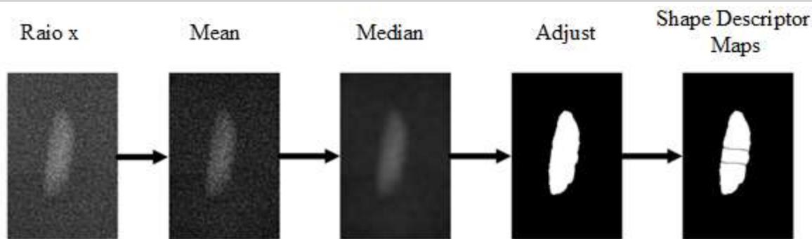
FIGURE 4. The sequence of the process of obtaining fissures in peellless rice through x-ray images.
