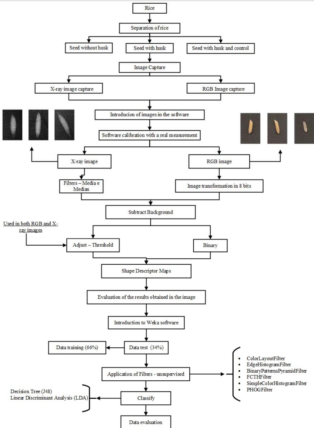
FIGURE 1. Schematic of X-ray and RGB image-processing for verification of cracks in rice seeds.
