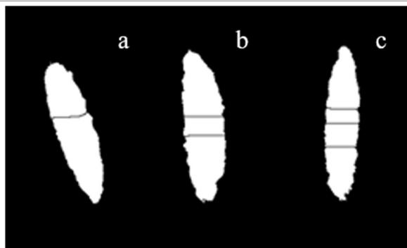
FIGURE 5. Fissures viewed after image processing in peeled rice seeds and dried captures by X-ray.
