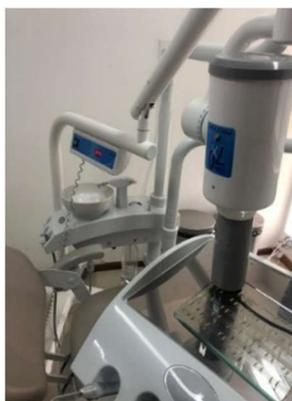
FIGURE 2. X-ray equipment and a sample of seeds on a glass plate.
