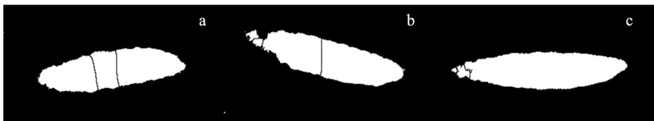
FIGURE 6. Fissures viewed after image processing in rice seeds with peel and without drying captured by X-ray, two fissures (a), one fissure(b), and no fissures (c), respectively.
