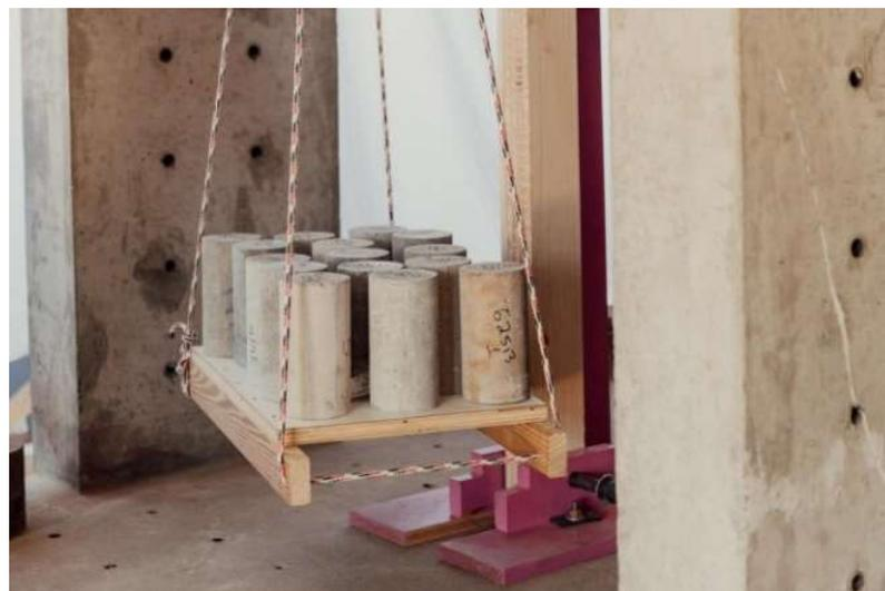
FIGURE 3. Tray with concrete specimens for structural loading.
