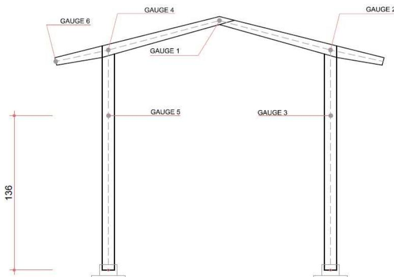
FIGURE 5. Arrangement of the dial gauges.
