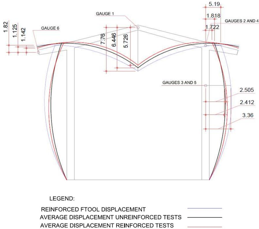
FIGURE 6. Comparison between the displacement estimated by Ftool, average displacements obtained from the unreinforced structures (Stringari et al., 2020), and with reinforcement, in mm, for design loading.
