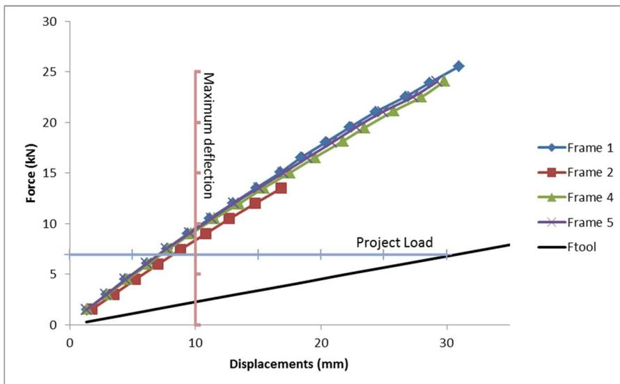
FIGURE 7. Force-displacement diagrams presented by Dial 1, ridge, without loading on the eaves.
