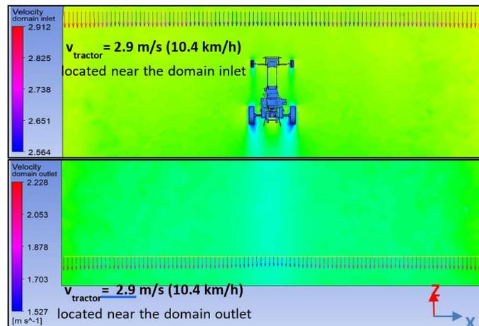
FIGURE 7. Velocity vector near the inlet and outlet of the flow domain at 10.4 km/h forward speed.
