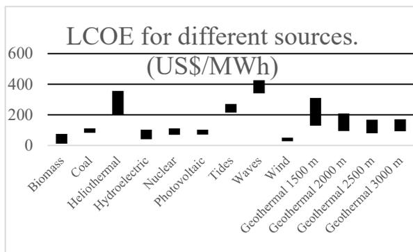
FIGURE 5. LCOE for different energy sources.
