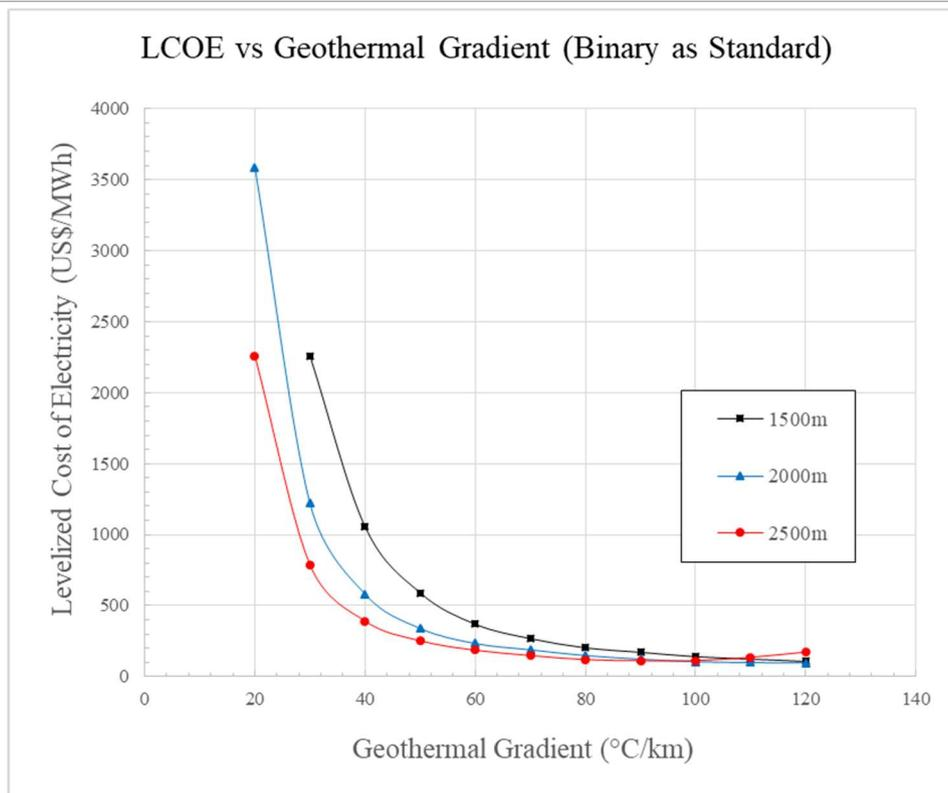
FIGURE 2. LCOE variation according to the geothermal gradient for binary power plants.
