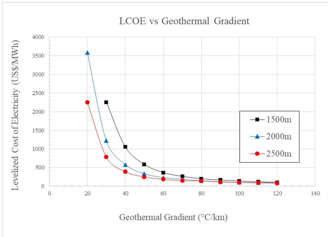
FIGURE 3. LCOE variation according to the geothermal gradient.
