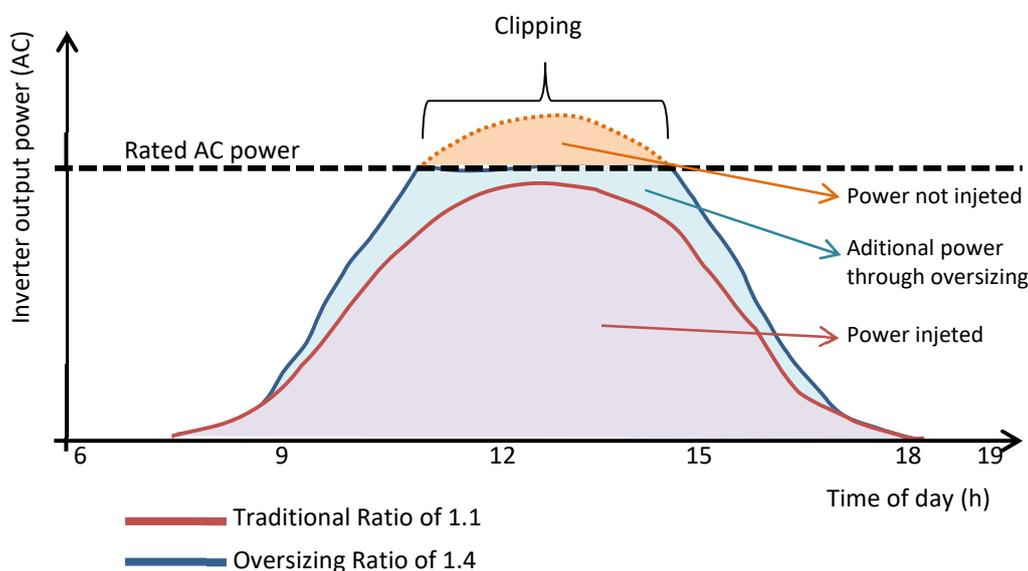
FIGURE 2. Oversizing and clipping on ten inverter samples. Source: Adapted from Souza (2019).
