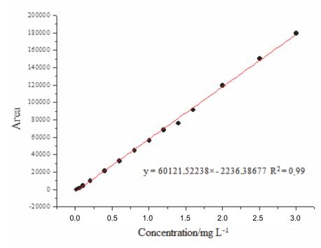
Figure 2 - Tebuthiuron calibration curve in CaCl, 0.01 mol L<sup>-1</sup>, obtained by high performance liquid chromatography.
