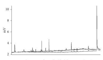
**Figure 4.** Gas chromatografic profile: black line is sample 3 (guava néctar of 14 °Brix) at time zero); gray line is 3-A sample (guava néctar of 14 °Brix) at 120 days stored at room temperature.
