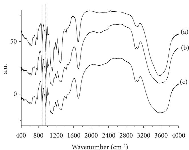
**Figure 1.** FTIR Spectra of (a)  $\kappa$ -carrageenan (b) commercial carrageenan and (c) native carrageenan.
