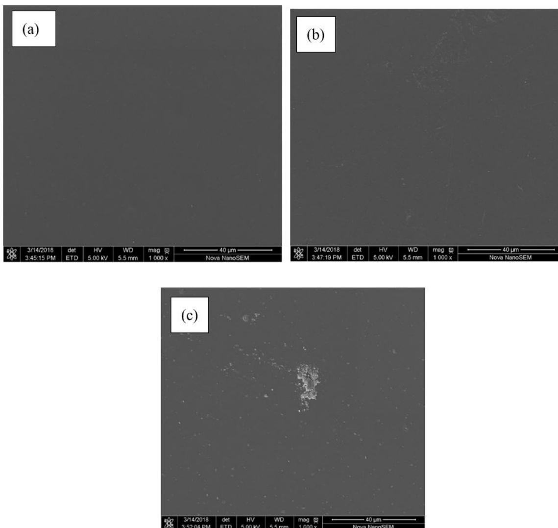
**Figure 1.** SEM of the surface for PVA film (a) and  $\epsilon$ -PL/PVA films with the  $\epsilon$ -PL content of 1% (b) and 5% (c).
