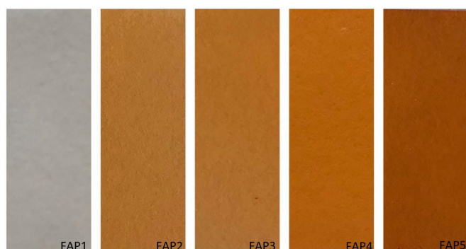
Figure 7. Arrowroot starch films incorporating EECC. FAP1: Arrowroot starch film with no EECC; FAP2: Arrowroot starch film with 0.25% EECC; FAP3: Arrowroot starch film with 0.50% EECC; FAP4: Arrowroot starch film with 0.75% EECC; FAP5: Arrowroot starch film with 1% EECC.
