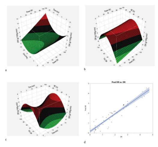
**Figure 2**. Response surface plots compare the drying rate of fenugreek leave influence by the interaction of time and power (a), power and moisture content (b), time and moisture content (c). While (d) represent the comparison of experimental and predicted value of drying rate.
