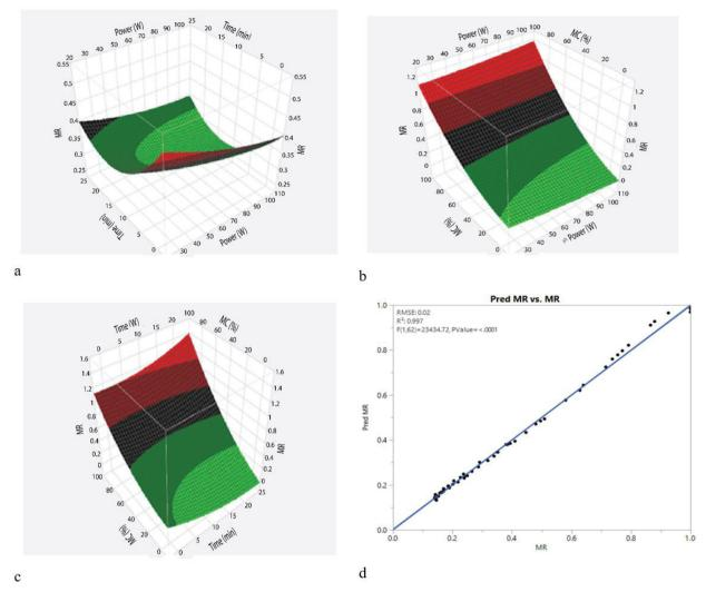
Figure 3. Response surface plots, moisture ratio as a function of time and power (a), moisture ratio as a function of power and moisture content (b), moisture ratio as function of time and moisture content (c), comparison of experimental and predicted moisture ratio (d).
