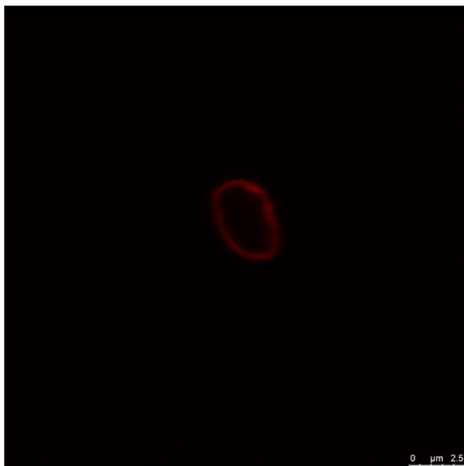
Figure 5. Confocal laser scanning micrographs of the W/O emulsion with the more stable formulation and stained with Rhodamine B. Source: own authorship.
