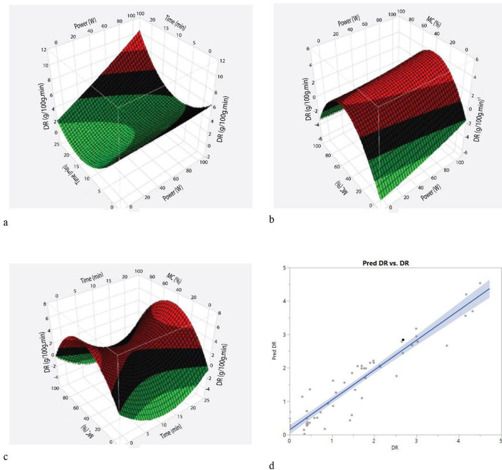
**Figure 2.** Response surface plots compare the drying rate of fenugreek leaf influence by the interaction of time and power (a), power and moisture content (b), time and moisture content (c). While (d) represent the comparison of experimental and predicted value of drying rate.
