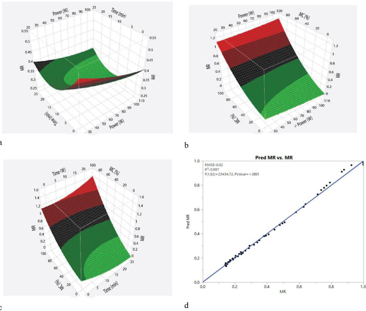
**Figure 3.** Response surface plots, moisture ratio as a function of time and power (a), moisture ratio as a function of power and moisture content (b), moisture ratio as function of time and moisture content (c), comparison of experimental and predicted moisture ratio (d).
